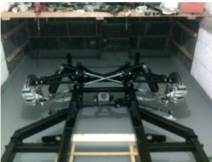
The front camber correction suspension
