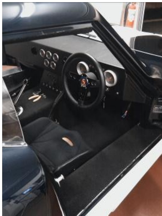
Insulation and carpet installation completed
