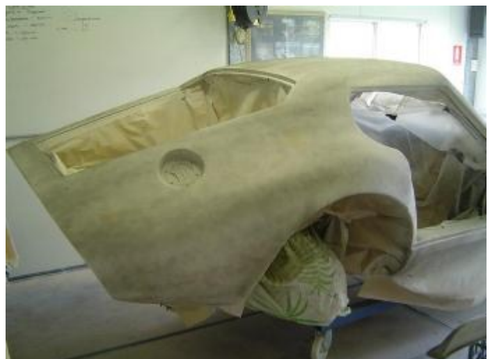
First spray putty and guide coat applied.
