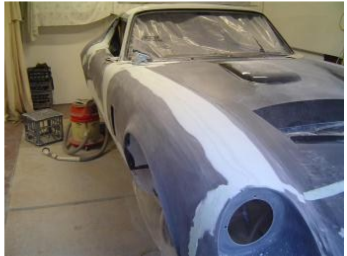
Drivers side nearing completion of filling and sanding stage
