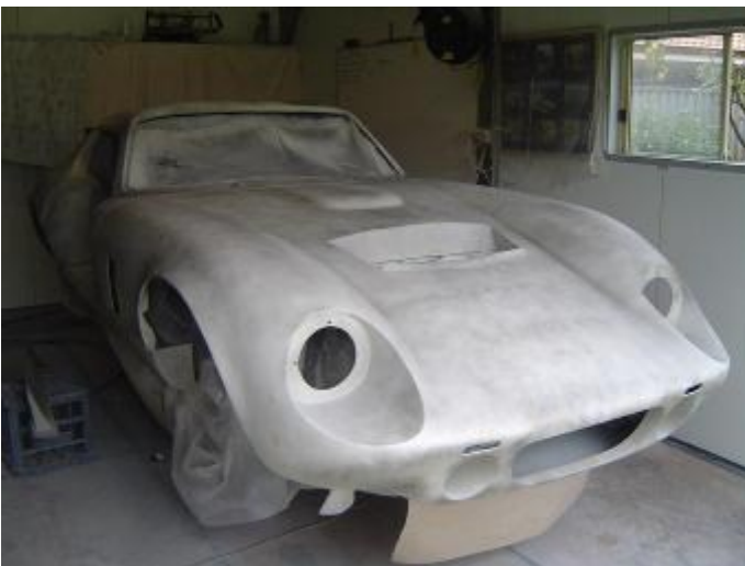
First spray putty and guide coat applied.
