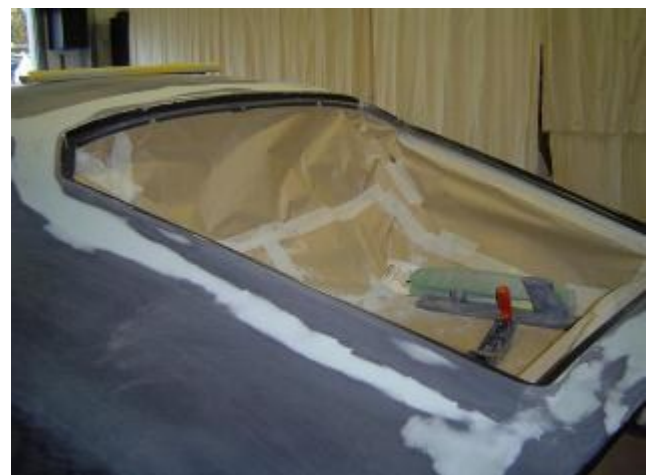
Correcting surface level around fuel filler recess and mould seams
