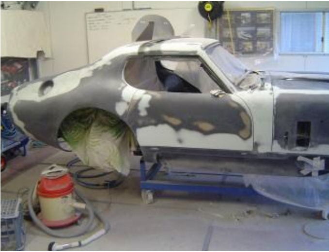
Drivers side nearing completion of filling and sanding stage
