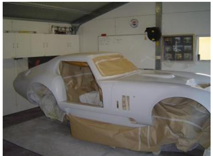
2 pack high build primer wet sanded ready for application of base colour
