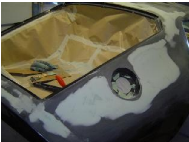
Correcting surface level around fuel filler recess and mould seams
