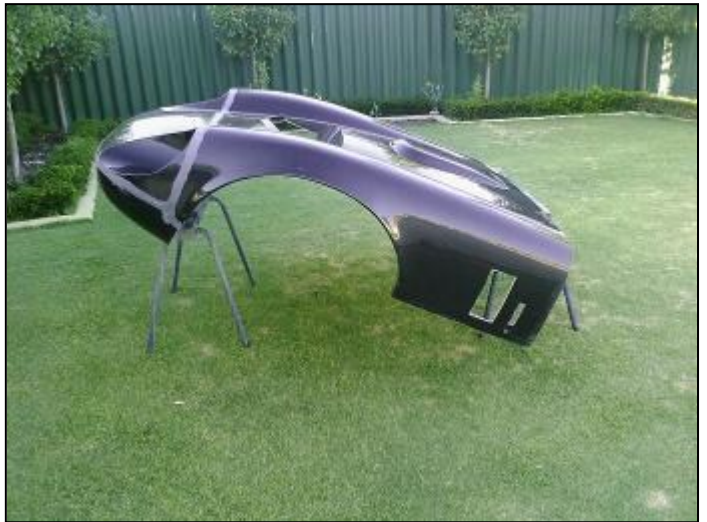
Front clip cut outs, mould seams cleaned up and wheel arch flange made uniform width. Ready for surface sanding.
