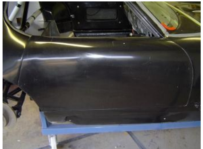
Main body and driver door installed
