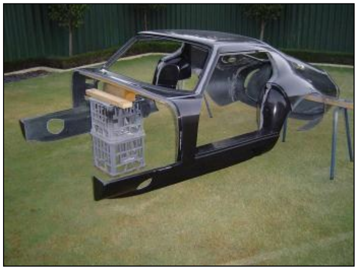
Front clip cut outs, mould seams cleaned up and wheel arch flange made uniform width. Ready for surface sanding.
