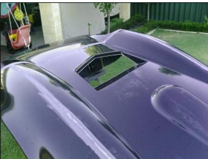
Front clip cut outs, mould seams cleaned up and wheel arch flange made uniform width. Ready for surface sanding.
