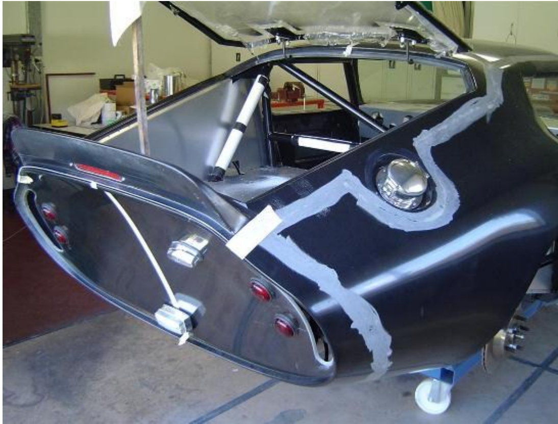
Rear lights, fuel filler and hatch all fitted (Note indicators to be changed to amber lenses)
