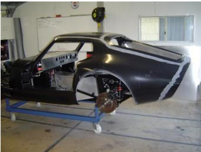
Main body and driver door installed
