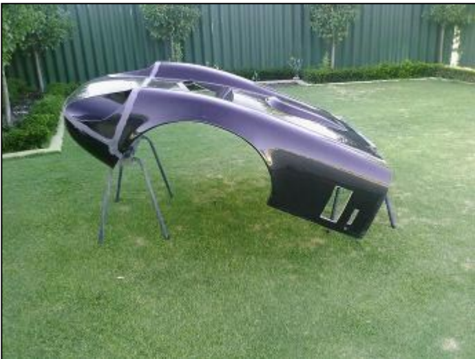
Front clip cut outs, mould seams cleaned up and wheel arch flange made uniform width. Ready for surface sanding.
