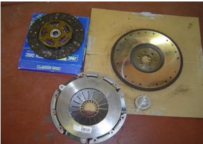
Engine rebuilt, Flywheel machined and new clutch components ready for installation
