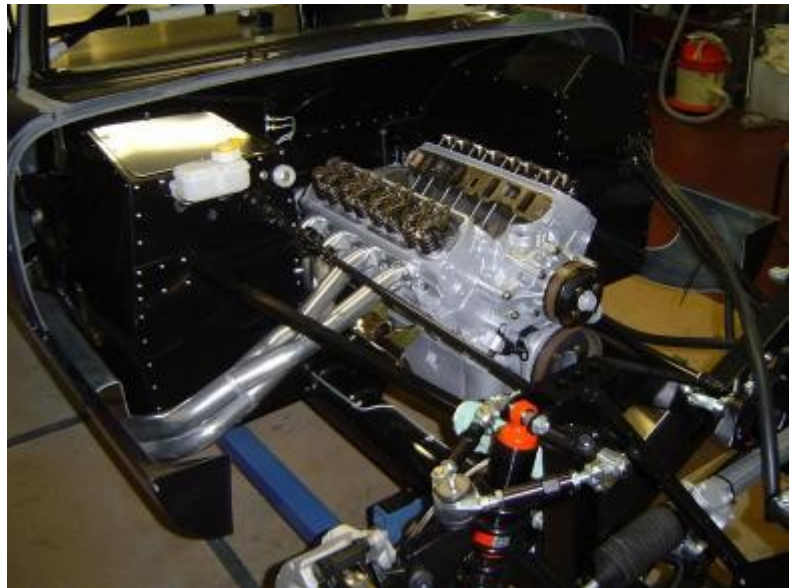
Engine and gear box installed with factory headers temporarily installed to check clearances
