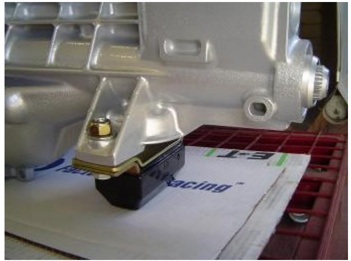
Gearbox mounting modified to clear chassis cross member and ready for install
