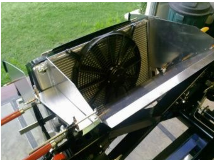
Radiator shrouding in progress.
