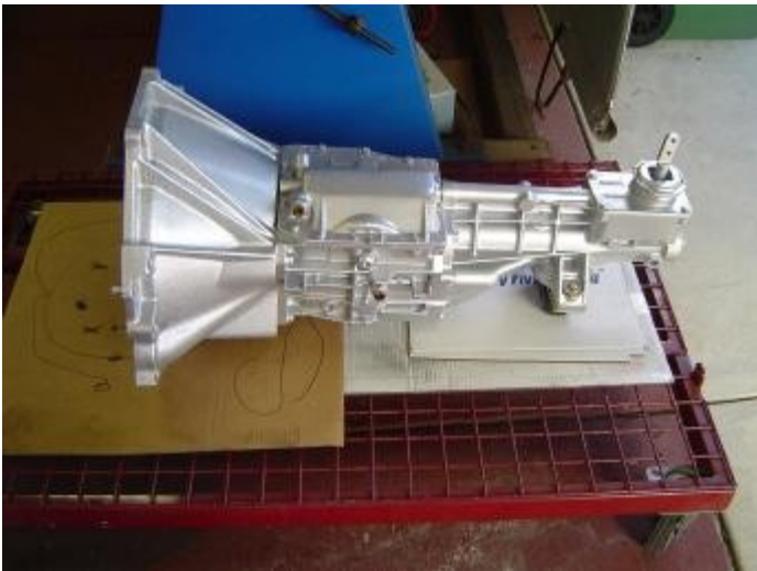
Gearbox mounting modified to clear chassis cross member and ready for install
