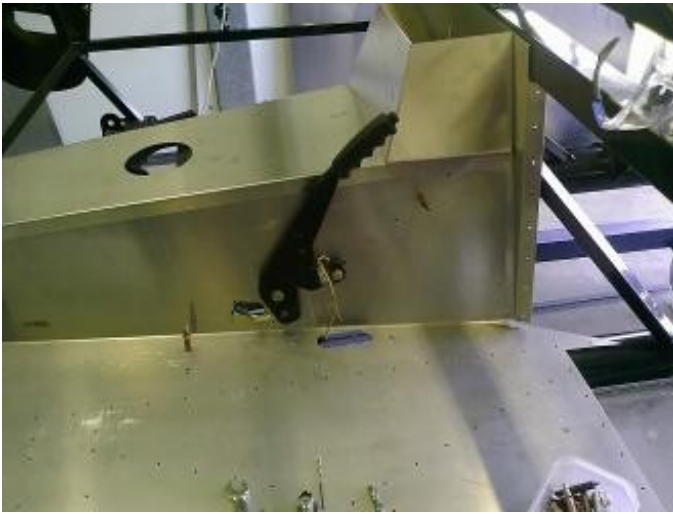
Handbrake installation test. Note cutout on floor for original FFR handbrake which positioned the hand brake way too far forward.
