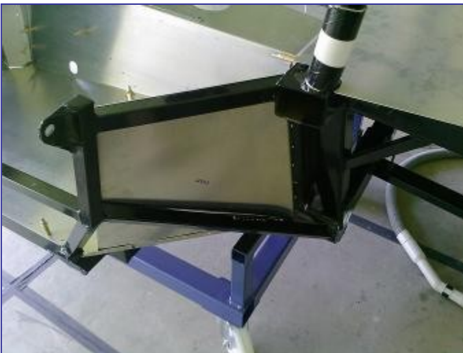
Rear splash panel refitted. Inertia reel seat belt mount bracket to be welded on and outer skin still to be fitted.
