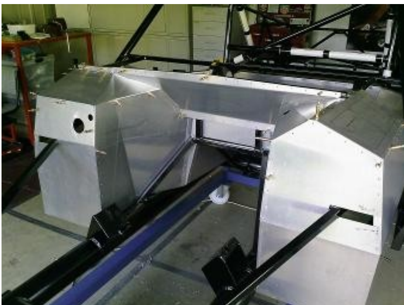
Rear splash panel refitted. Inertia reel seat belt mount bracket to be welded on and outer skin still to be fitted.
