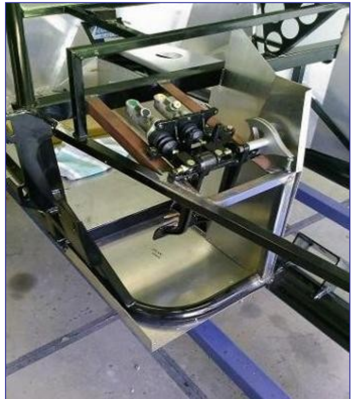
Pedal box mounting and steering column fitment in progress
