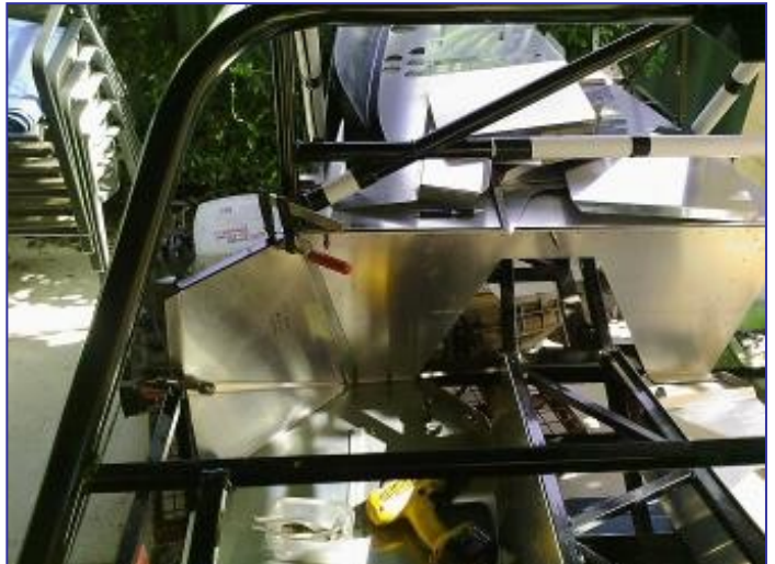
Fitting up rear bulkhead panel and re-bending to fit chassis properly
