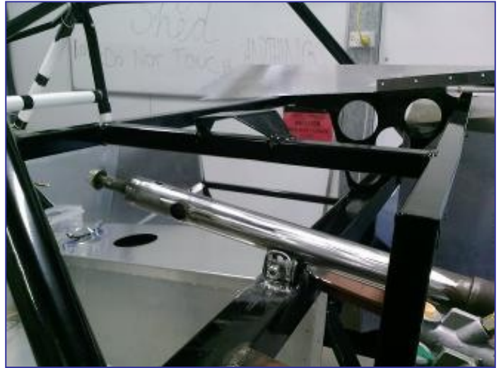
Pedal box mounting and steering column fitment in progress
