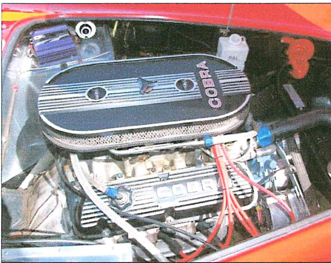
Joe Craig's 302 cu/ins Boss Mustang engine
